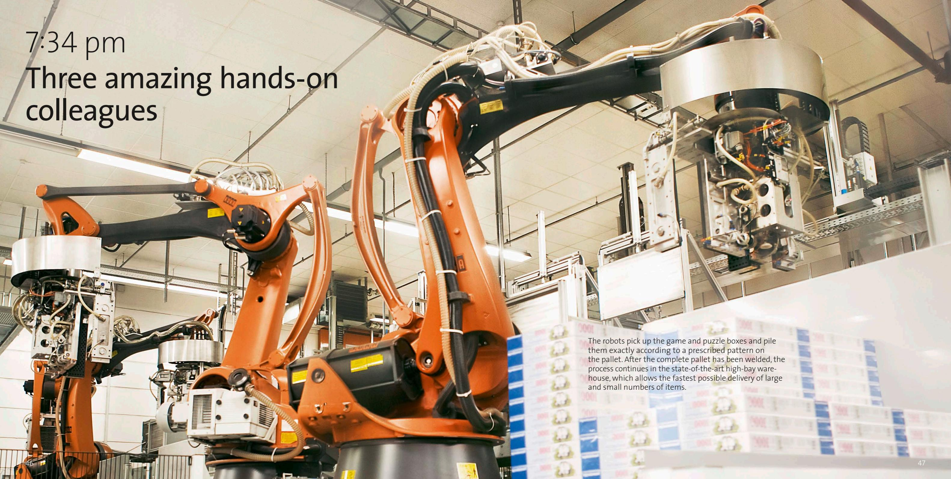
The robots pick up the game and puzzle boxes and pile them exactly according to a prescribed pattern on the pallet. After the complete pallet has been welded, the process continues in the state-of-the-art high-bay warehouse, which allows the fastest possible delivery of large and small numbers of items.
